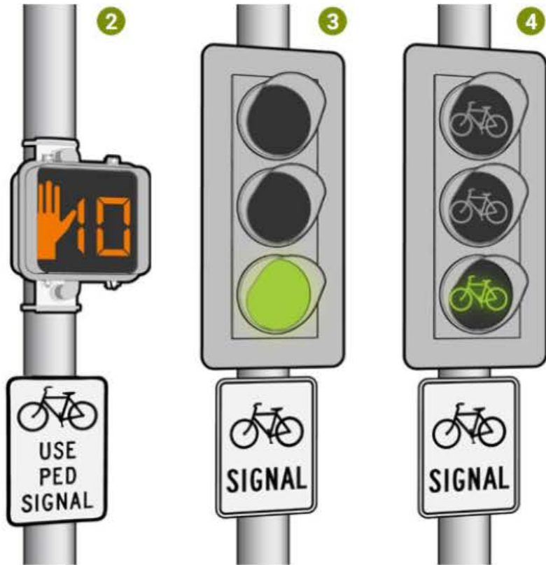
Figure 10.14. Examples of Signal Indication Strategies for Bicyclists
