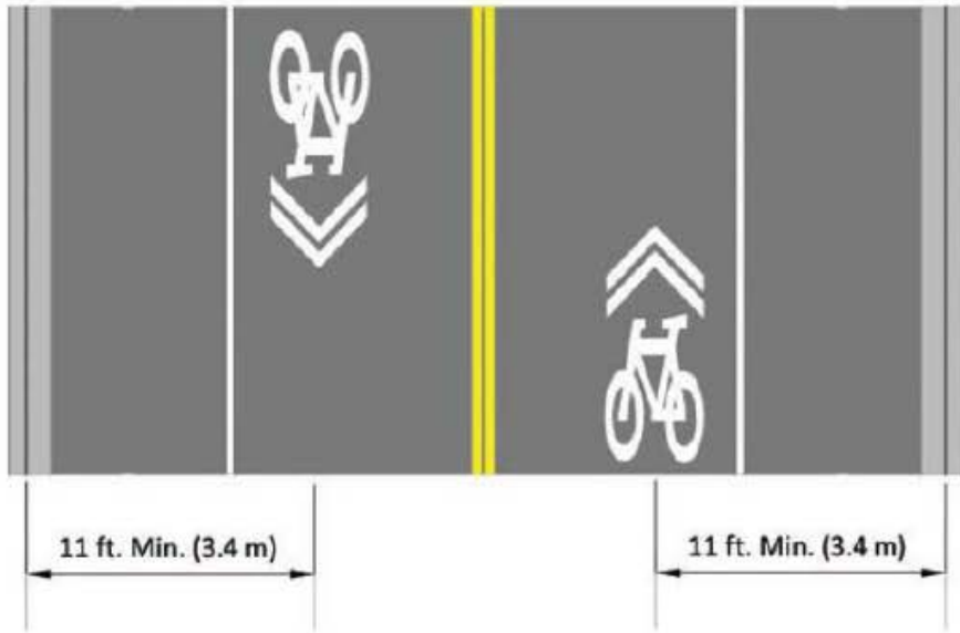
Figure 4-5. Typical Shared-Lane Marking Cross Section on Street with Parking
